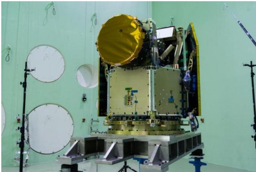
The CHEOPS spacecraft on a ground support structure inside the Large European Acoustic Facility
